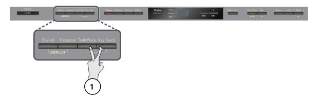
1. Hold down the [Twin Piano] button and press the [Key Touch] button.
